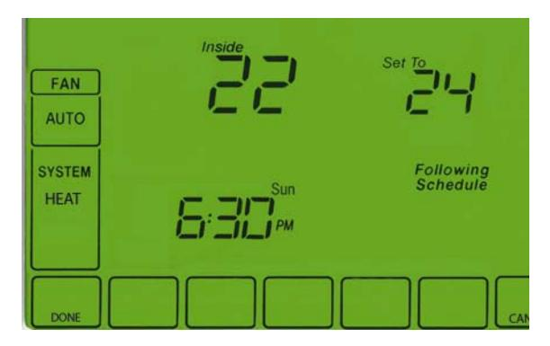
2. Temporarily set the temperature to higher than the current room temperature (example 24°C). "WAIT" will show in the lower right just below "SET TO" temperature display.
